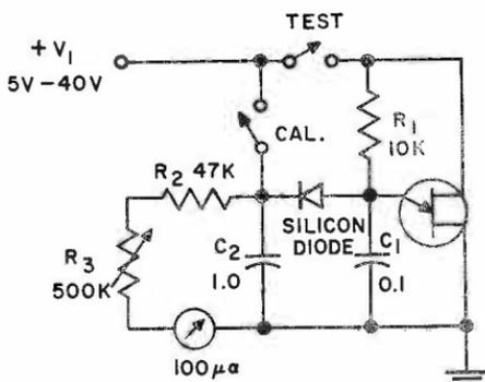
TEST CIRCUIT FOR INTRINSIC STANDOFF RATIO ( $\eta$ )
