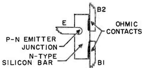
Construction of unijunction transistor—cross sectional view
