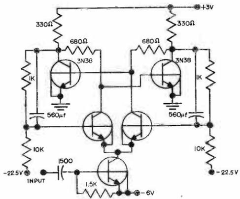
CIRCUIT OF FIGURE 126 (b) WITH TRIGGER STEERING ADDED FOR COUNTER APPLICATION
