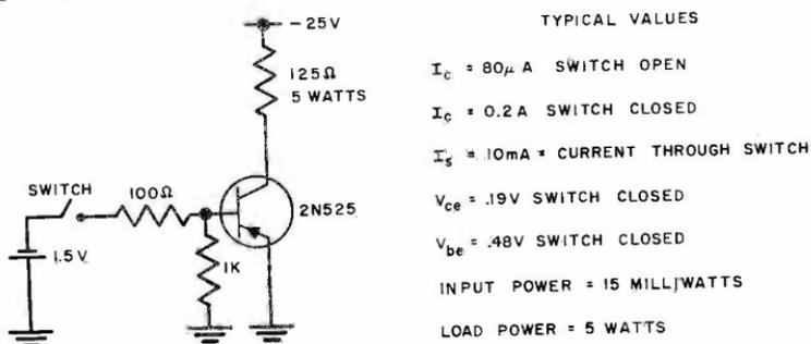
Typical transistor switch application
