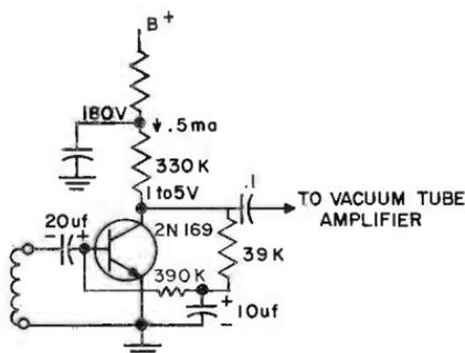
NPN PREAMPLIFIER FOR MAGNETIC PICKUPS
