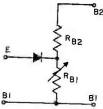
Unijunction transistor representative circuit
