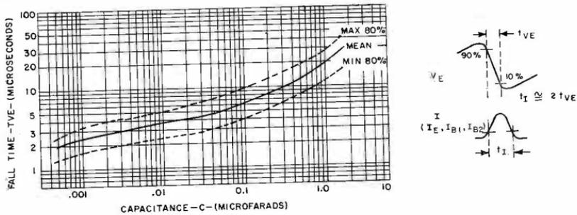
Recovery time of unijunction transistor relaxation oscillator vs. capacity
