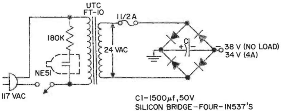
POWER SUPPLY FOR DUAL SIX-WATT AMPLIFIER
