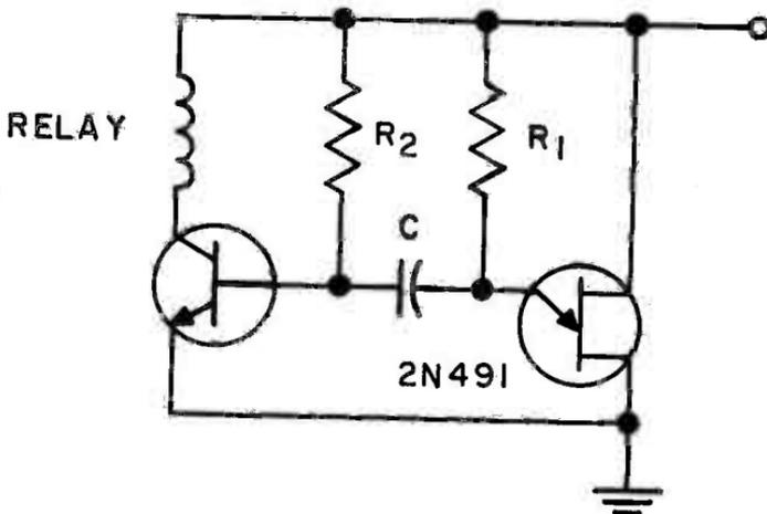
Unijunction transistor multivibrator used to drive NPN transistor
