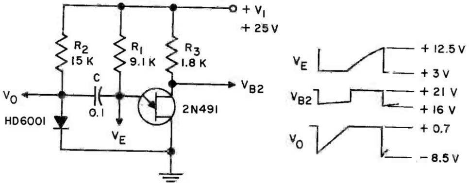
UNIUNJUNCTION TRANSISTOR MULTIVIBRATOR
