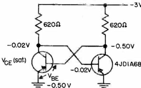
DIRECT COUPLED TRANSISTOR LOGIC (DCTL) FLIP-FLOP
