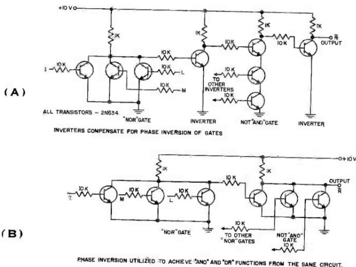
Circuits representing  $(I + M + L) (\bar{I} + \bar{M} + \bar{L}) (\bar{I} + \bar{M} + L) = \bar{R}$
