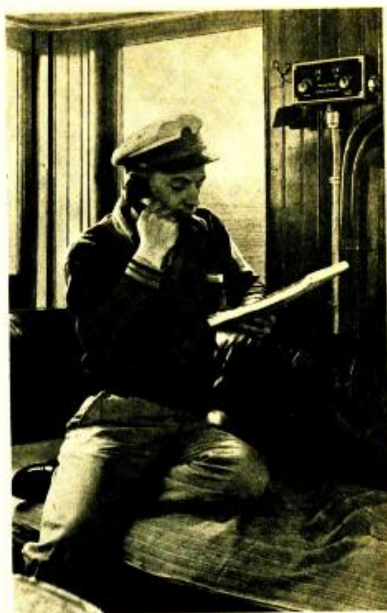
Capt. Woelfffing of the pilot steamer "Sandy Hook" can keep in touch with shore or other ships by means of the new marine radio telephone equipment. The shore operator can ring the bell in the wheelhouse. (Photo courtesy Western Electric Co.)
