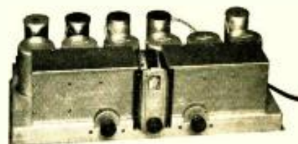
Fig. 1. A band-selector tuner manufactured in 1929, for high-fidelity broadcast reception. It was known as the "MB-30."
