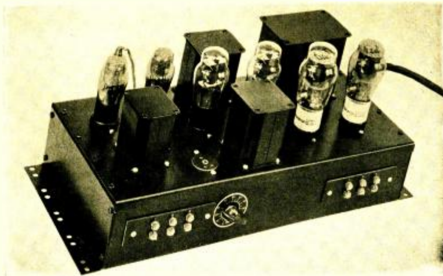
View of the complete driver amplifier, with inverse feedback, which employs type 1608 tubes in the output.
