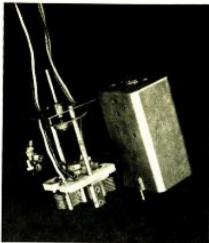
Fig. 7. Close-up of one of the "fixed-tuned circuits" removed from its shield can. Note variable air trimmers and mechanism for altering coupling between the coils. This is a standard commercial type i.f. transformer.
